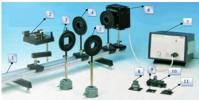
Figure 5.19 Investigation of the coherence of light with spectral lines using the Michelson interferometer Specifications
