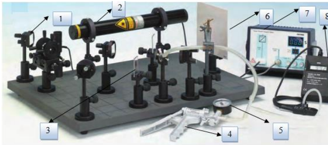
Figure 5.21 Determination of air refraction index using Maha-Zhender interferometer Specifications
