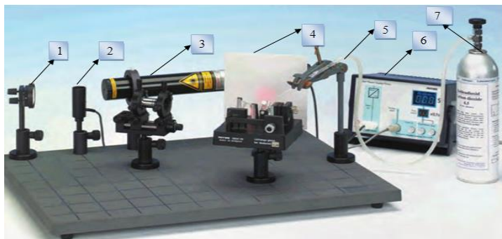
Figure 5.20 Determination of the CO 2 index using the Michelson interferometer Specifications
