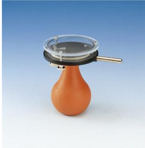
Figure 8.24 Detection of radioactive radiation with the Wilson cloud chamber
