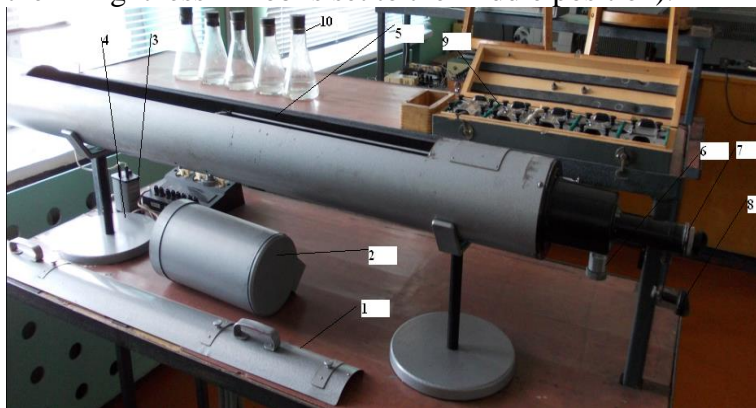
Figure 5.61 General view of the interferometer ITR - 1 - upper cover; 2 - protective cap; 3 - transformer T-4; 4 - stands; 5 - thermostat; 6 - a drum with a scale; 7 - line pipe; 8 - magnifier; 9 - set of ditch; 10 - solutions for the experiment
