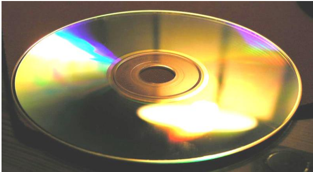
Figure 6.47 The laser shines through the «back» of a compact disk. The grooves in the disk act as a diffraction grating, producing a spectrum
